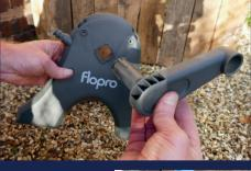
Align the drum and insert the central plastic winding handle through the hole in the frame and into the drum
