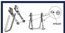
Build the lower frame and secure with 4 x screws ST5x20
