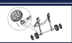
Push on the wheels and click into place the outer wheel trim on each side
